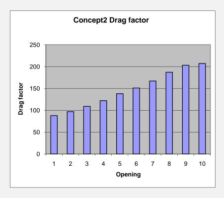
The bar chart shows a slight nonlinearity between these quantities but this can be the result of inaccuracies in the setting of the inlet slide.
