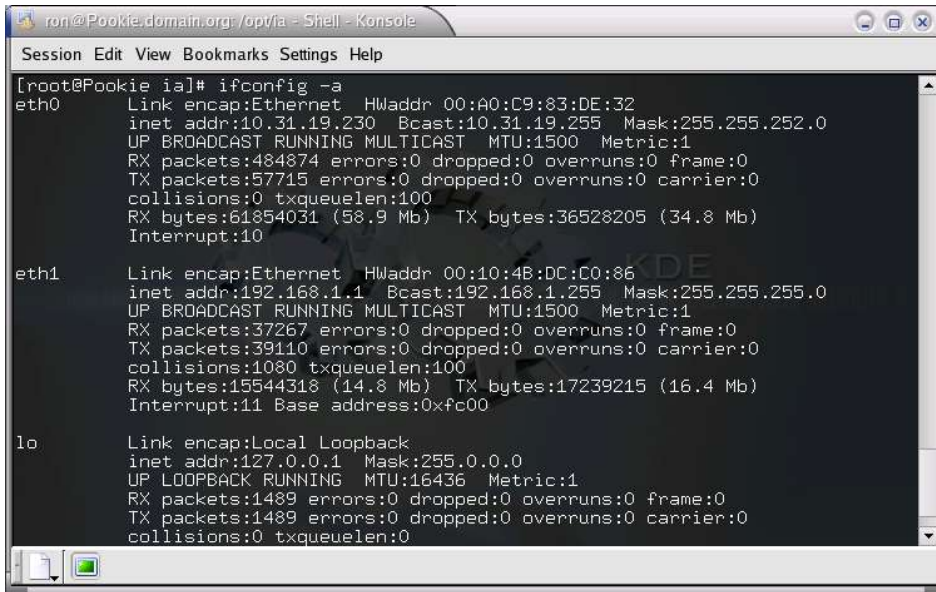
Illustration 14 On the Linux box: results from "ifconfig -a" command As we can see (we are primarily interested in the eth1 card), the network is configured with IP address 192.168.1.1/255.255.255.0 . (Note the hardware address as we will use that in the dhcpd.conf file to force that IP address to this interface). The eth0 network interface was, in our configuration, connected to the office network. We used that to obtain data from the outside world. It is of no real importance to our task here.
