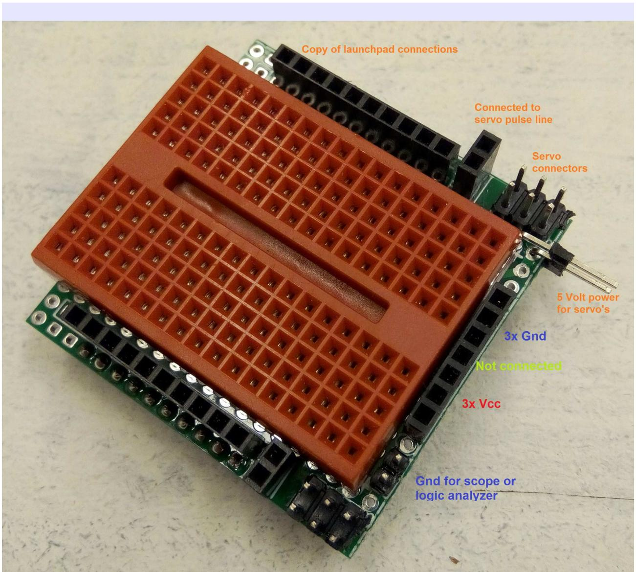
Purpose of connectors on top side of finished Egel shield
