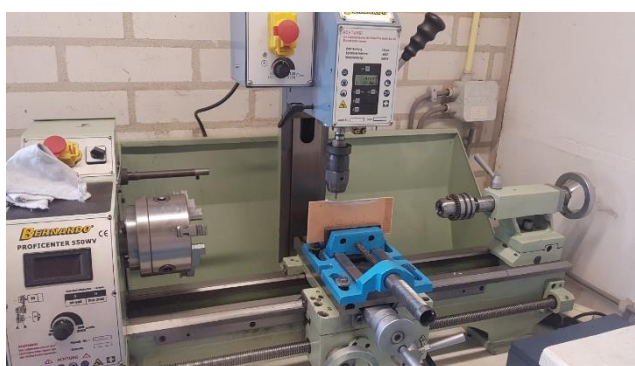
Photo 4 : Measuring on the milling column, with 0.01mm resolution
