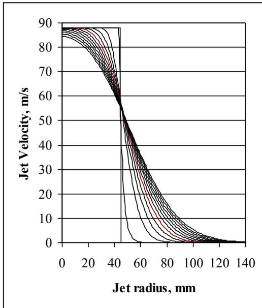
Figure 23 Velocity profiles, mass ratio=1.8
