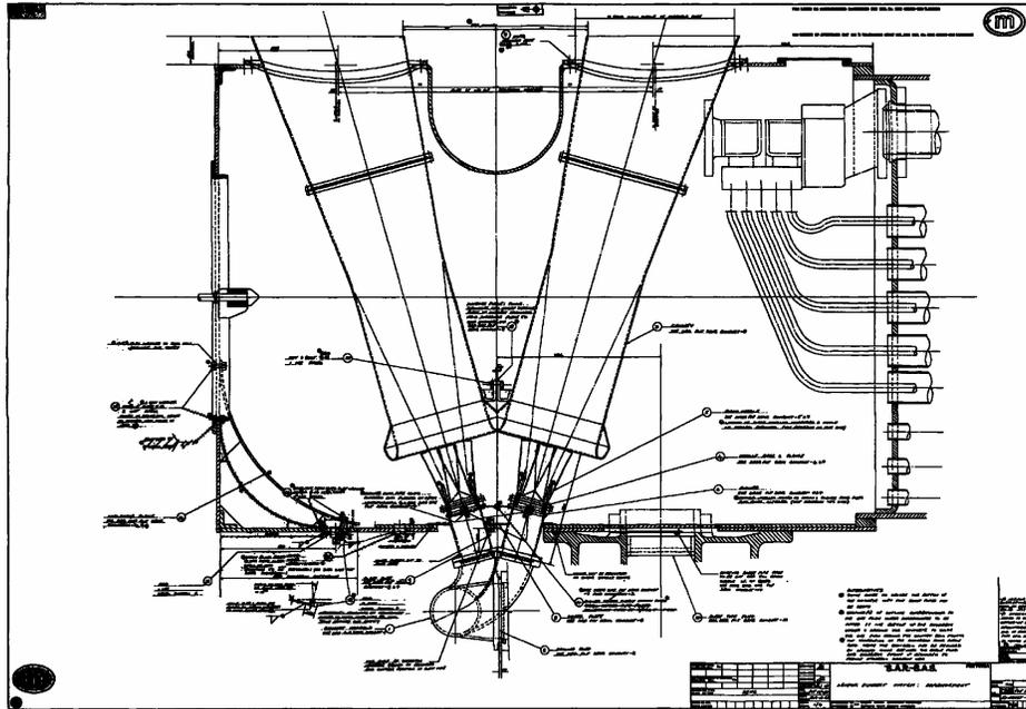
Figure 18 SAR 26 Lempor exhaust system by Wardale<sup>23</sup>
