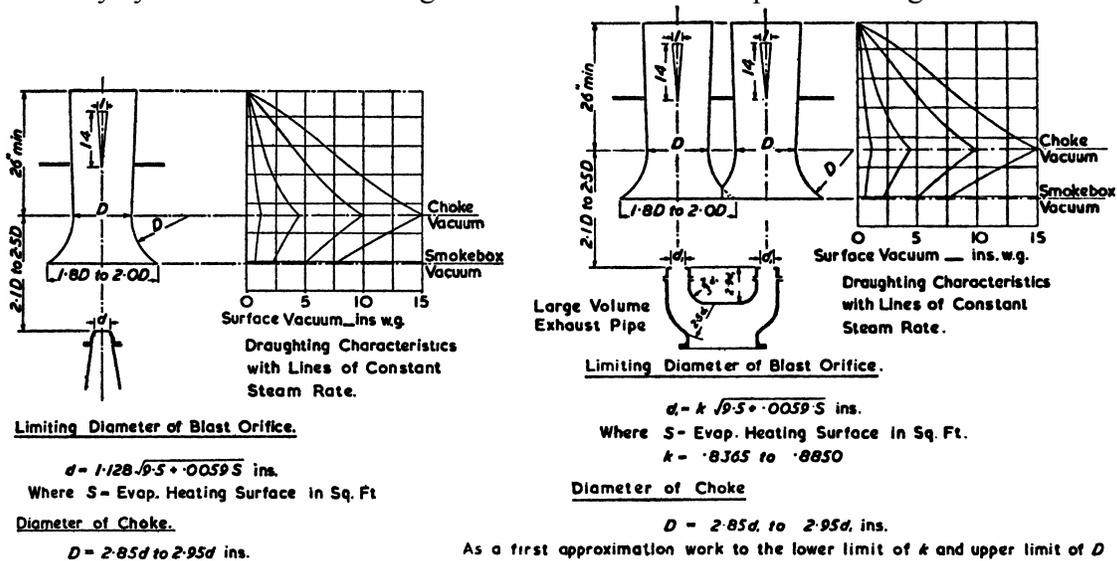
Figure 17 Front-end dimensions according to Ell<sup>21</sup>
