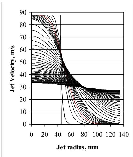
Figure 25 Velocity profiles, mass ratio =3.02
