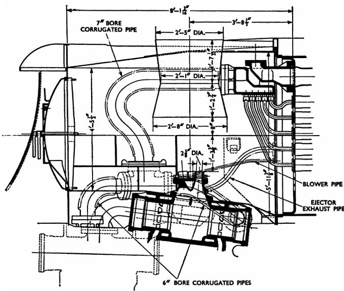
Fig. 267.—" Merchant Navy " class; cross-section of smokebox.
