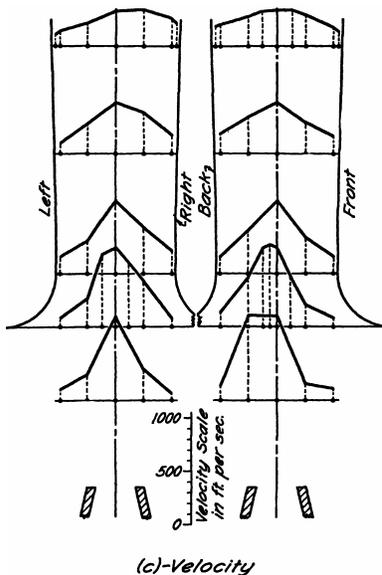
Figure 28 is taken from Young<sup>32</sup> and shows the measured velocity distribution, in two directions, of his 1:4 front end model. It shows the same type of velocity distribution development as discussed earlier.
