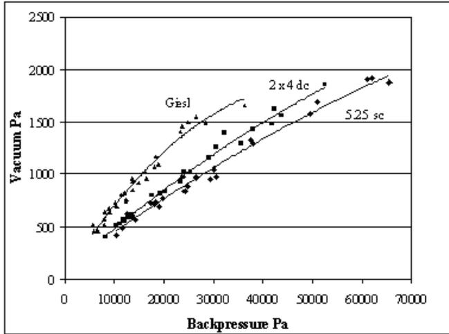
The vacuum curve for the Giesl shows very good performance at the lighter loads but tends to curve to the right at the higher loads. This indicates an asymptotic approach to a limit. This was designed on purpose as described by Slezak in his book on the Giesl Ejector<sup>20</sup>
