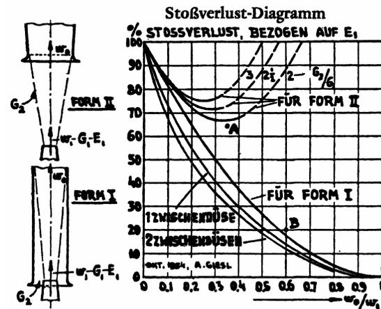
Figure 14 Giesl-Gieslingen shock loss diagram<sup>18</sup>
