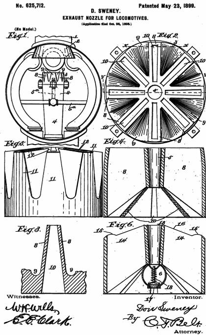
Figure 5 Sweney patent drawing<sup>6</sup>
