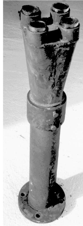
Figure 31 Blast pipe with 4-orifice blast cap
