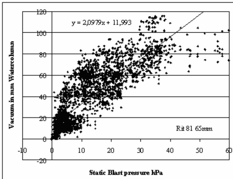
Figure 32 RTM 54 test, results of the original 65 mm orifice
