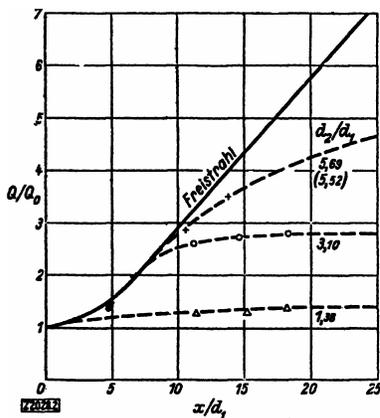
The results are shown in Figure 22 They clearly show almost identical results as those of Zeuner: the ratio of total mass  $Q$  to that of the driving fluid mass  $Q_0$  cannot be larger than the ratio of the catching tube to orifice diameter would allow for.
