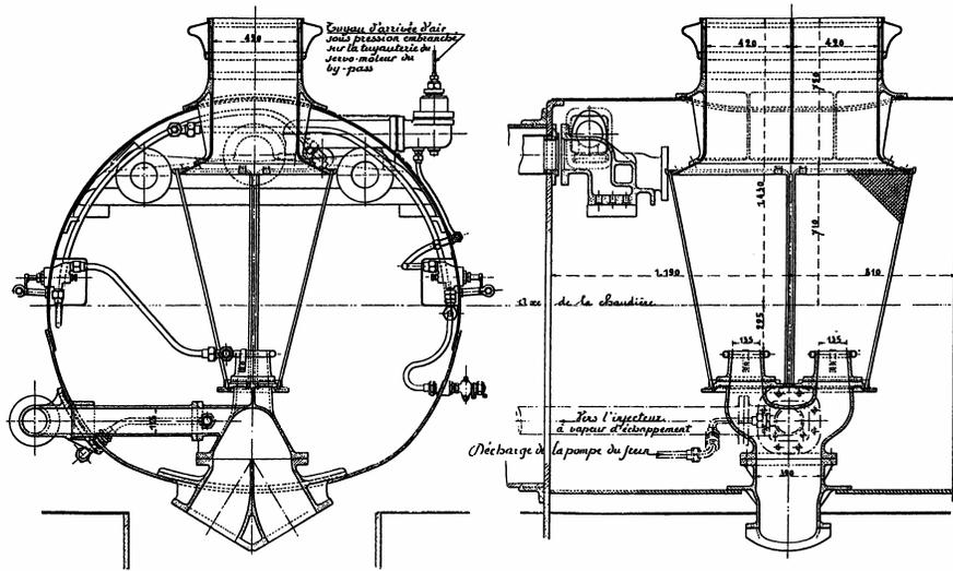
Figure 7 Belgian Railways Pacific type 10 with double chimney<sup>8</sup>
