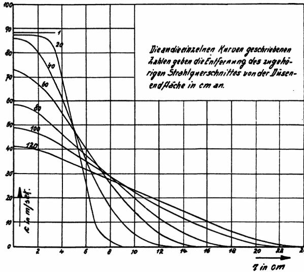
Figure 20 Velocity profiles as measure by Trüpel<sup>26</sup>
