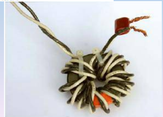
Fig 30 – A line filter for 1-14 MHz
